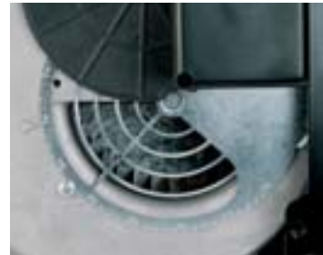
Air damper completely open (GS10, GS20)
