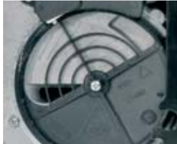
Air damper partially open (GS3, GS5)
